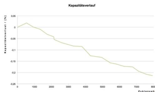
The AKAMODULE 46Ah still has 80 percent of its original capacity after over 8,000 full load cycles. (Photo: AKASOL)
