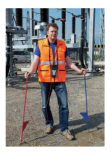
Preliminary location with shirla narrows sheath faults down to a few meters. With the step voltage method and the corresponding manual devices, pinpointing the exact position is easily performed.
