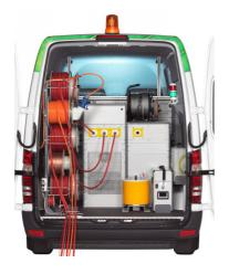
The new 3.5 tonne BAUR cable test van also enables automated cable testing, diagnostics and fault location up to 80 kV, and provides a wealth of new functions with version 3.3 of the BAUR system software.
