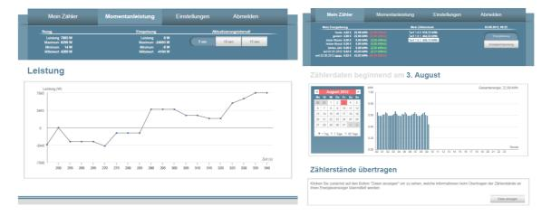
The Smart Grid Hub's built-in web server allows the consumer's usage figures to be displayed and analysed on the computer without any need for the data to go beyond the house.
