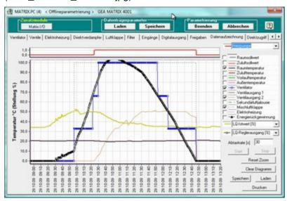
The new GEA MATRIX control system matches the air flow to the measured values reported by a CO<sub>2</sub> or mixed-gas sensor.
