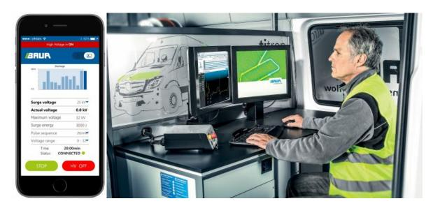
Remote control via app: The surge voltage generator of the titron cable test van can be started and stopped for the cable fault pin-pointing via the smartphone. This way, the cable route is not loaded with high voltage pulses for longer than necessary.
