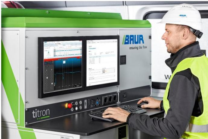
Parallelised processes – such as the combination of dissipation factor and partial discharge measurement into a single sequence – speed up measurement tasks. Measurement engineers are thus able to collect significantly more information and generate additional benefits for asset and maintenance management. To get the most out of the information, standard processes
