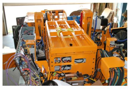
Stable and safe storage for underground use in harsh conditions: the AKASOL AKASYSTEM 15 AKM NMC NANO lithium-ion battery system. (Photo: Medatech)
